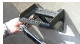
6. Position step iron anchor and tighten with a torque wrench with T_{inst} = 25 \text{ Nm} .
