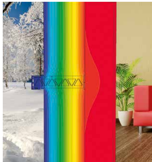
Image 2 Minimal thermal bridge with CROSSFIX®
