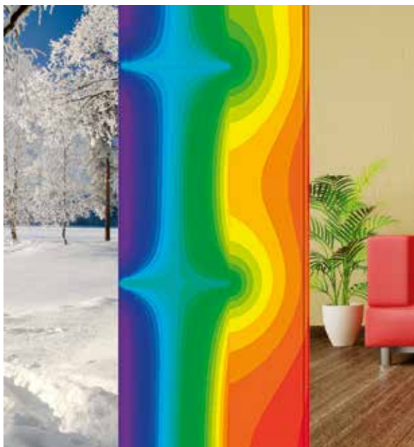
Image 1 Pronounced thermal bridge on aluminum consoles
